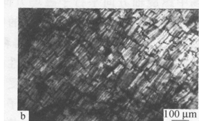
Fig. 3 Effect of magnetic field on the fingerprint texture of the EC/DCA cholesteric solution: micrographs of high (a) and low (b) magnification
